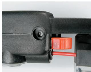
**Adjustable drive roll tension** for feeding different types of wire.
